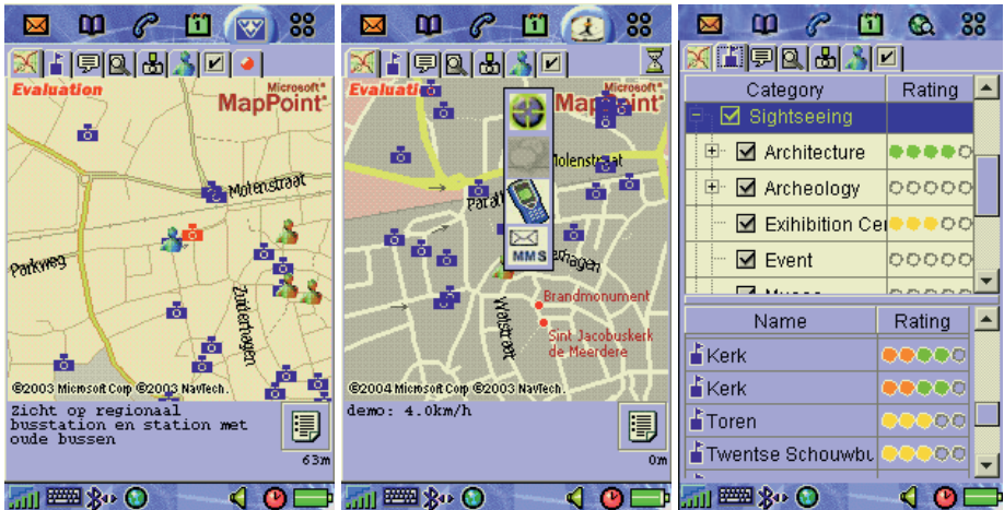
Fig. 1. Screenshots of the COMPASS application: objects near the user on the map, interacting with services offered by objects and a list of objects near the user with relevance scores.
